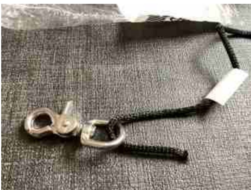
Figure 4 Snap hook, line and heat shrink tubing
