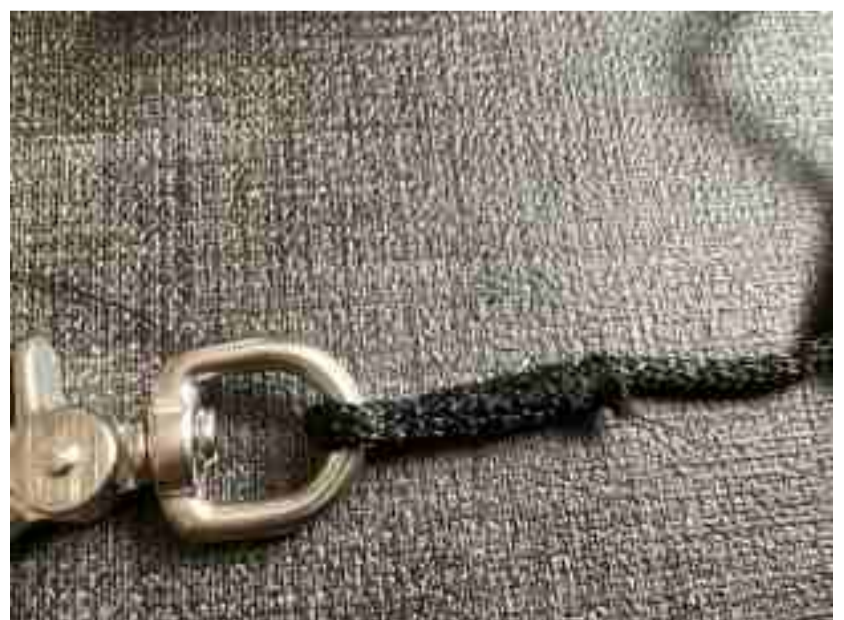
Figure 5 Snap hook attached with sewn eye
