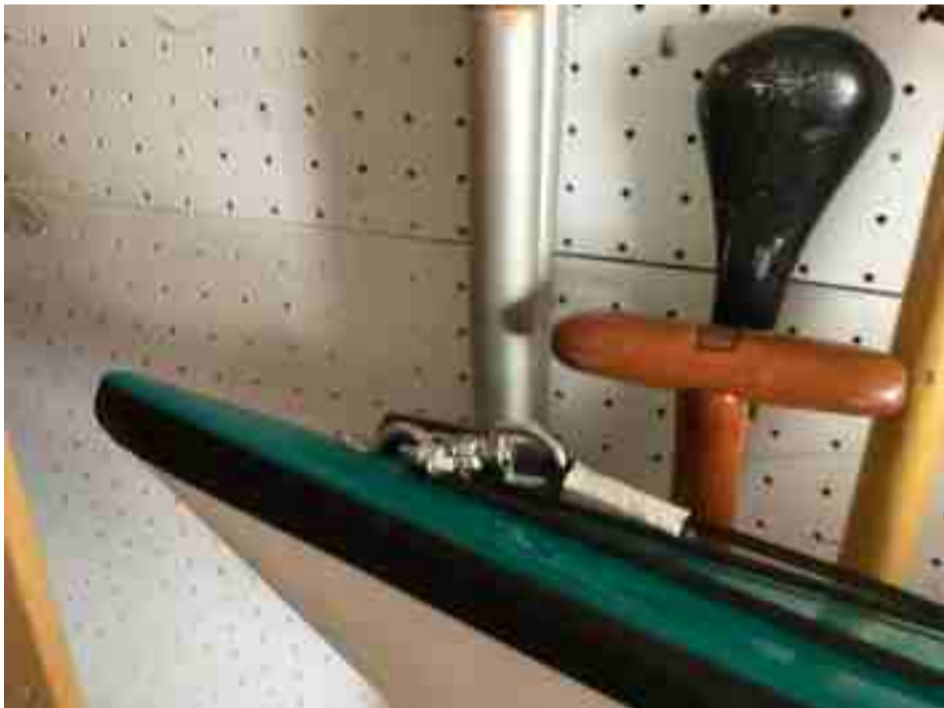
Figure 8 Snap hook attached to fixed metal loop on bow
