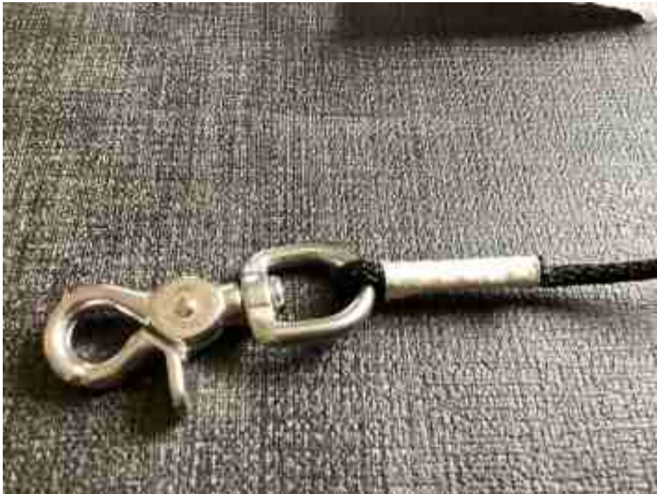
Figure 7 Snap hook attached with sewn eye covered by heat shrink tubing gloves.
