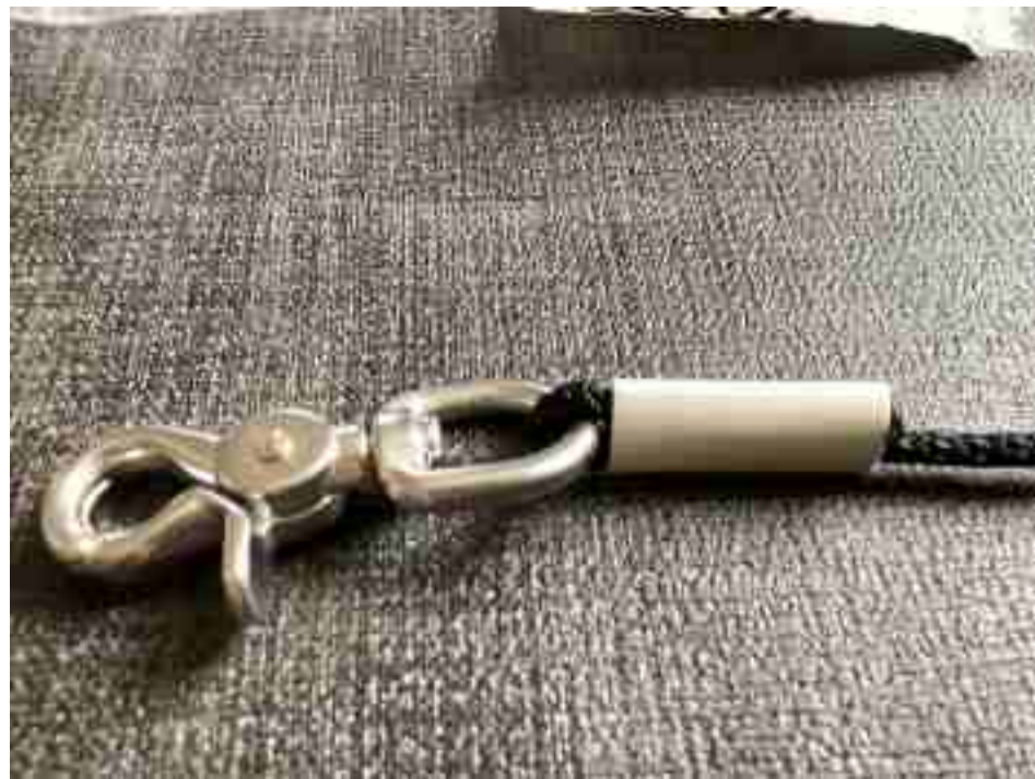
Figure 6 Heat Shrink slipped over sew eye shank
