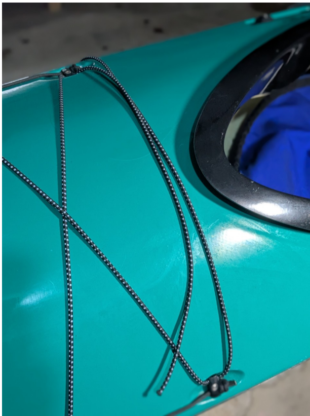
Fore deck pattern before tying grapevine knot (double fisherman's bend)
