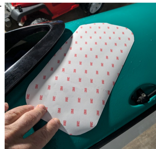
3M paint protection film being fitted. The backing peels off and you spray a water-soap slip fluid to position the film and squeegee out air bubbles.
