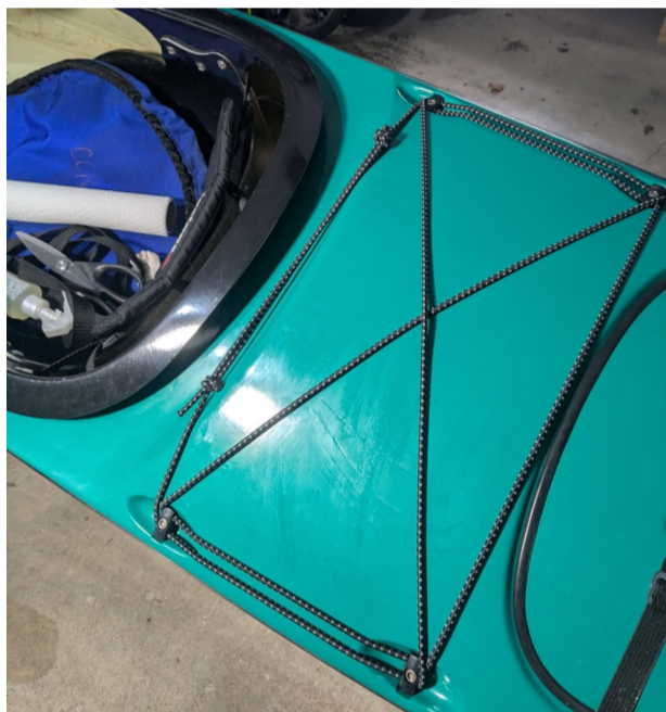
Aft deck bungee complete with grapevine knot. Note double bungee at deck edges.
